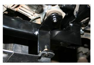
8. Attach mud flap using M6 roof bolt and nut.
